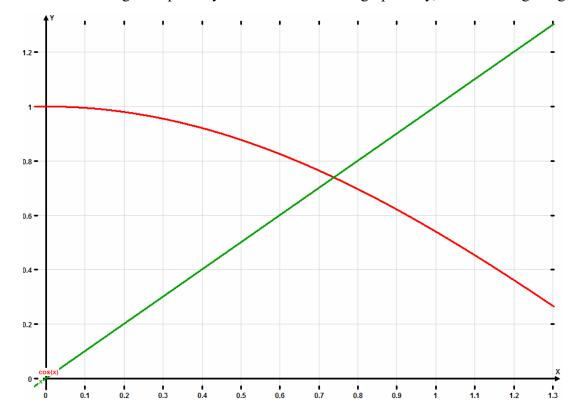
From that point on the x-axis. travel vertically up until the line touches the g(x) $= \cos x \text{ line. Then,}$ travel horizontally, and where it crosses the y-axis is where  $g(x_2)$  is. From there, go horizontally to the left, and it will cross the y = x line. When a straight line is drawn directly from that point to the x-axis, the new point on the xaxis will be the value of x2. This can then be repeated continuously until it touches the fixed point. When the graph
