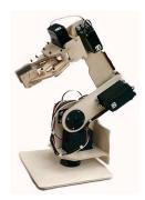
Servo controlled robots are used for sensing their own positions and feeding back the sensed position to the control, and they do this in a way in which the control causes a particular path to be followed. A non servo robot has no way of determining if they have or have not reached a specific point and acts out a task blindly.
