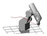
If a robot is able to move from one specified point to another, but is unable to stop at arbinary points that have not been previously designated, then this is called a point-to-point robot. Point-to-point robots that are driven by servos are often controlled by potentiometers and/or limit switches, which is set to stop the robot arm at a specific point.
