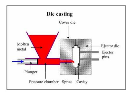
This level of versatility has placed die castings among the highest volume products made in the metalworking industry. In recent years, injection-molded plastic parts have replaced some die castings because they are cheaper and lighter. Plastic parts are a practical alternative if hardness is not required and little strength is needed.
