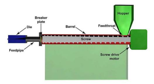
In the extrusion of plastics, raw thermoplastic material in the form of small beads (often called resin in the industry) is gravity fed from a top mounted hopper into the barrel of the extruder. Additives such as colorants and UV inhibitors (in either liquid or pellet form) are often used and can be mixed into the resin prior to arriving at the hopper.
