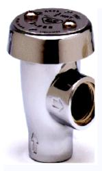
An Atmospheric Vacuum Breaker (AVB) is a backflow prevention device used in plumbing to prevent backflow of non-drinking liquids into my drinking water system. It is usually constructed of brass and resembles a 90 degree elbow with a hood on its top to allow air to enter the water system if a siphon attempts to form. On the left is a photograph of a typical Atmospheric Vacuum Breaker.
