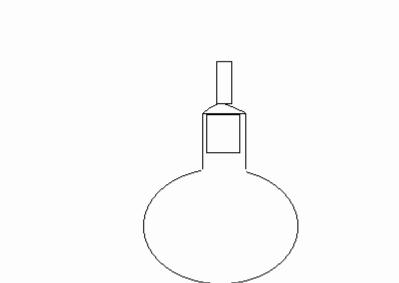
Fig 1. Pycnometer design
