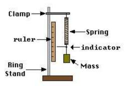
I performed this experiment to determine how the extension of a spring varies with the stretching force. A spring is hung vertically from a fixed point and a force is applied in stages by hanging weights from the spring. The apparatus is set up as shown above. For the purpose of the experiment I used different gram 50 to 400 gram, and the extension of the spring I measured it metres.
