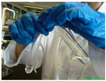
5. All the test-tubes were standed in the beaker and heated to  $60^{\circ}$ C. Then, the Bunsen burner was removed.
