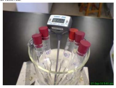
6. 1cm³ of aqueous silver nitrate was quickly added to each of the tubes A to D and the stopclock was started. Each tube was shake once to mix the contents, and was leaved in the water with the cork resting loosely on the tube to reduce evaporation.
