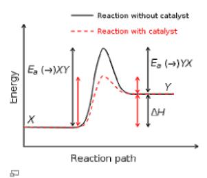
Generic potential energy diagram showing the effect of a catalyst in an hypothetical exothermic chemical reaction. The presence of the catalyst opens a different reaction pathway (shown in red) with a lower activation energy. The final result and the overall thermodynamics are the same.
